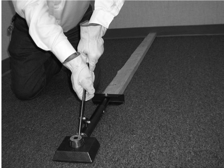
When extension support is required, we recommend the use of a 2 x 4 stud as shown in the photo above.
