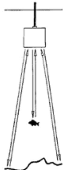
6. The Transducer can be used directly in the water to look for Fish, but the Display unit should never be immersed.
