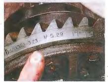
OEM gears and most aftermarket sets are marked at the ring gear with the gear ratio. Our 8.75 featured 3.23:1 gears, which is the most common ratio found in muscle car–era Mopars.
