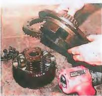
We opened our Sure Grip for inspection by removing the eight housing bolts. The Auburn design uses cone clutches behind the side gears, which engage the differential housing. This design is very effective and durable, but can eventually wear out.
