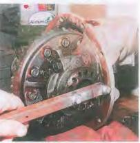
The third member was moved to the vice bench for full teardown and inspection. Step one is removing the carrier. We backed off one main cap fastener to reduce the tension on the spanner adjusters, and then backed the adjusters off to relieve the carrier bearing preload using a homemade spanner tool.
