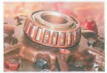
While assembled, the gear chunk looked great, but once inside the carrier bearings told a different tale. These bearings are clearly dead, as evidenced by readily apparent rust and pitting. A more common sign of wear is fine radial grooving along the rollers, also evident on our bearings.
