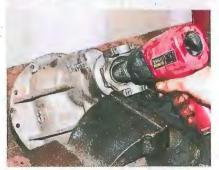
Back at the gear chunk, the pinion nut and yoke are removed to release the pinion. Since this is a #489 case housing, the pinion uses a crush sleeve to set the pinion bearing preload. Removing the yoke means the crush sleeve will need to be replaced upon reassembly.
