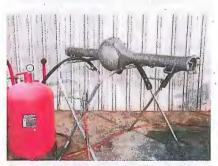
Our rear housing was sandblasted to white metal using a Harbor Freight pressure pot sand blaster and #30 mesh silica sand. The insides were then cleaned with solvent followed by serious scrubbing with detergent and brushes, and then blown dry. This part is now ready for paint.
