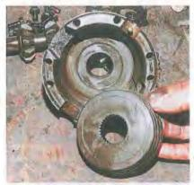
As the cone clutch wears, it goes deeper in the housing, and eventually bottoms, no longer providing any grip. Our clutches were just starting to bottom, as we could see by the clear contact pattern on the cone face. This Sure Grip differential is essentially done, though it could be revived by machining the cones for added clearance and adding spacer shims behind the side gear. We will likely replace the unit.
