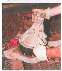
The center gear chunk is the business end of an 8.75-inch rear, and it drops out with 10 bolts once the axleshafts are clear. Placing the rear in an upright position will prevent spilling a mess of hypoid lube once the chunk is broken loose.
