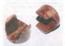
Our differential coughed up a broken thrust block (spacer) when removed. The thrust block normally surrounds the differential pinion shaft, and requires disassembling the Sure Grip unit to replace. Its purpose is to work with the axleshaft adjuster to set the endplay with tapered roller bearings, but it is not necessary with replacement "green" style bearings.
