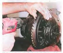
Make sure to mark the main caps so that they can be reinstalled in the same position, and then remove the cap fasteners to pull the carrier andring gear. Our Harbor Freight Earthquake air impact wrench can handle tough bolts with ease.
