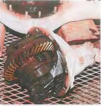
Inside our gear chunk looked good, preserved by a healthy coating of gear lube. The bonus was finding a factory Auburn Sure Grip limited-slip differential. While we seemed to be in luck with the limited slip, these cone-clutch Sure Grip units do eventually wear out.
