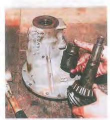
Usually a few blows with a softfaced mallet at the end of the pinion is all that is required to free it from the front pinion bearing and allow the pinion to drop out of the case. The crush sleeve arrangement is not an optimal setup for performance use, but it can be replaced with a solid spacer and shims when a major service is being performed.
