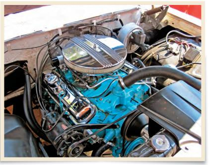
♦As it sits, the Catalina is equipped with a 303hp, 389ci V-8 backed by a fatally wounded Jet-Áway Hydromatic transmission. The 303hp four-barrelequipped 389 had been rebuilt in the recent past and will benefit from the new Turbo Hydromatic in its future.
