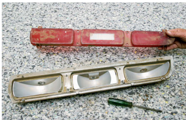
Our lenses and housings were in exceptional shape and just needed cleaning and polishing. Rougher examples will need abrasive blasting and refinishing of the bright silver reflective paint inside the housings.
