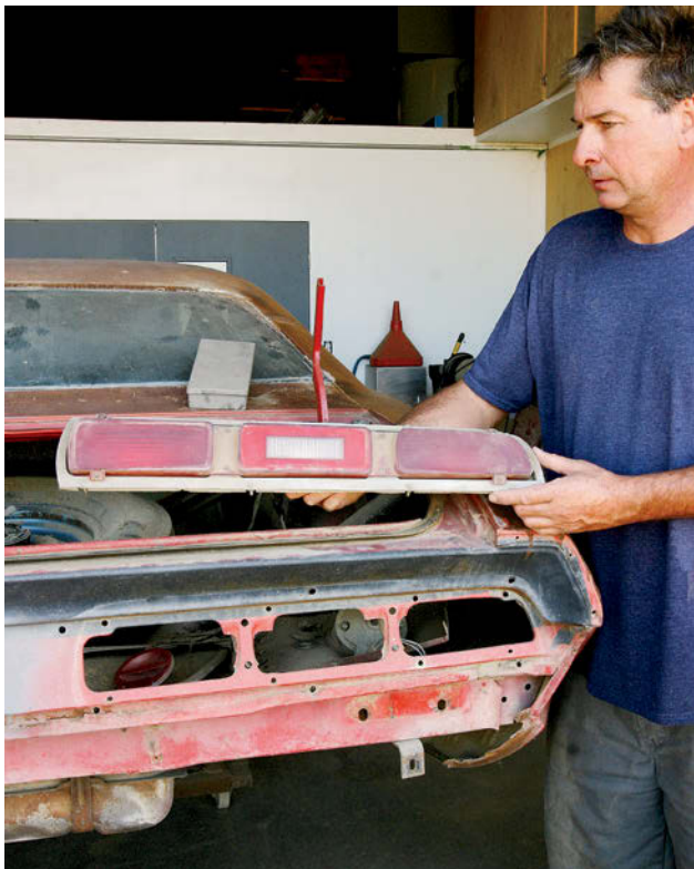
The taillamp housings and the trim bezel are completely separate assemblies. The trim panel unbolts from inside the trunk, and once removed the taillamp housings and lenses can be unbolted and removed. The bulb sockets are integral with the rear wiring harness and simply pull out of the taillamp housings.
