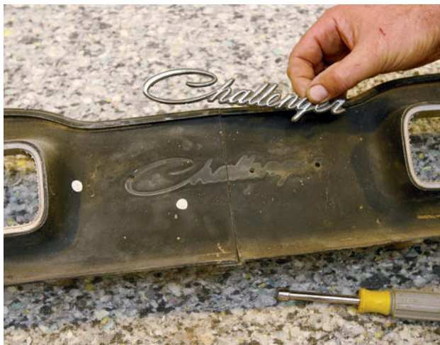
The trim panel is actually made up of two separate pieces that overlap and attached in the center via two delicate peened attachments. When off the car these can easily break, which will undoubtedly fracture the Challenger script emblem that bridges the two. Ours survived intact, and even the Challenger emblem was in very nice condition.
