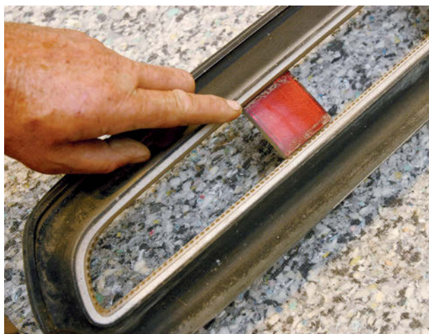
The trim panel simply overlays the taillamp lenses, and features four delicate reflectors built into the framework, which give the illusion of full-width taillamps, even though the lenses actually have three distinct segments. It is a very unusual arrangement.
