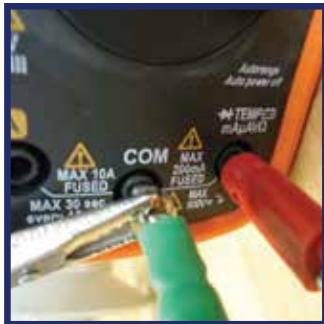
Test Setup Connected To + V and Com
