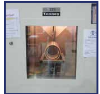
Tumbler in Environmental Chamber During Testing
